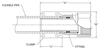
P-Series fitting to be used only for P-Series pipe.
