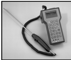
Model PTE-1 with HQS-RT1 and RTD Probe installed
