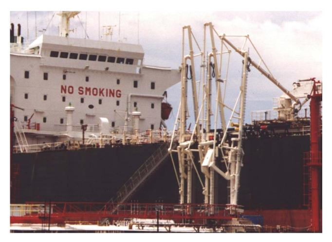
The B0030 Marine Loading Arm is preferred when loading/unloading sea-going tanker ships and its capability has been proven within many years of trouble free operation world-wide.
