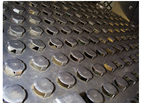
Figure 4. MINIVALVE Deck - Floating Valves
