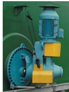
fig.8: Mechanical Actuator on Gear Mixer
