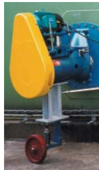
fig.9: Castor Support on Belt Mixer
