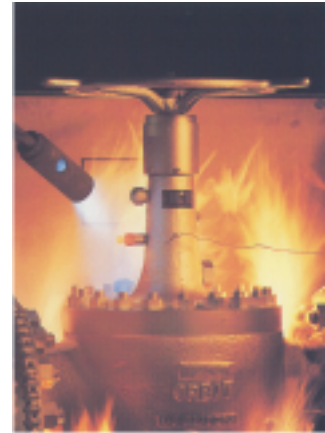
Fire Testing and Certification to the latest industry standards is performed under the eye of independent inspectors.
