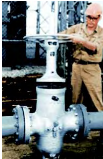
Technician demonstrating bonnet removal and in-line repair of WKM Model E
