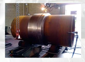
PIPELINE INSULATING JOINT are used worldwide for permanently controlling the flow of electrical currents or electrically isolating pipe sections in pipes and piping systems. Effective management of cathodic protection programs results from the use of these highly reliable substitutes for flanged insulating systems.
