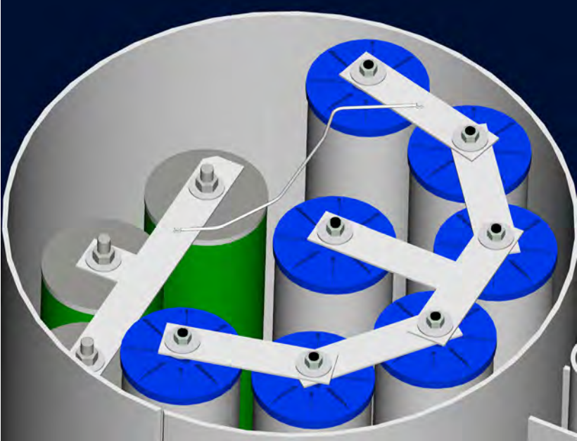
Figure 2. Two spiders in vertical filter/separator bonded together with braided stainless steel wire, bonded to vessel via separator tie-rods.
