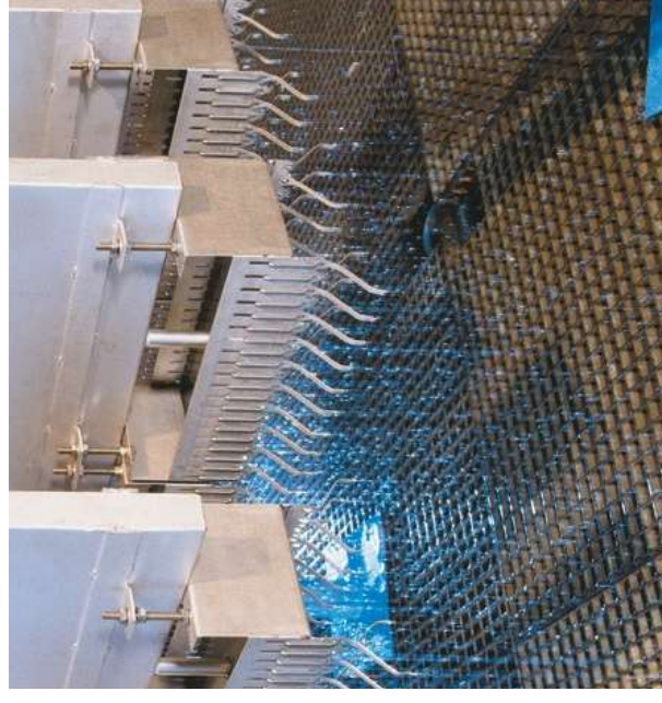
The liquid distributor Type S shown here is one example of a solution to a customer's problem for distributing small volumes of liquid
