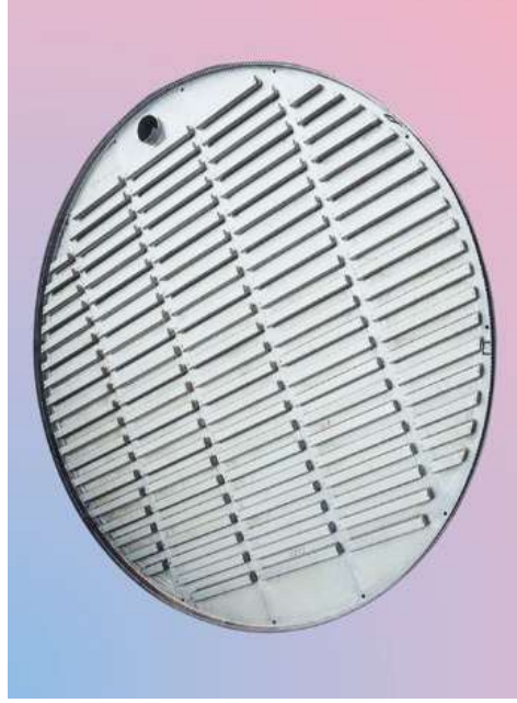
Thormann® tray DN 3400 mm, one piece, made of titanium. This tray is of a leakproof design and is intended for use in an HCl-absorption column made of GHP.
