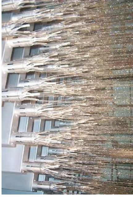
Montz liquid distributor Type S with short drip fingers
