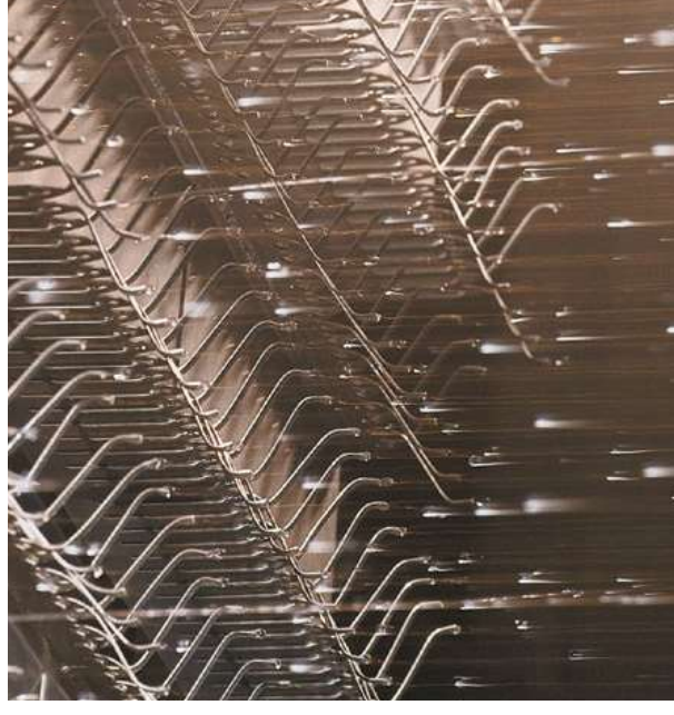
▶ Drip pattern of a Montz liquid distributor Type S (special design)
