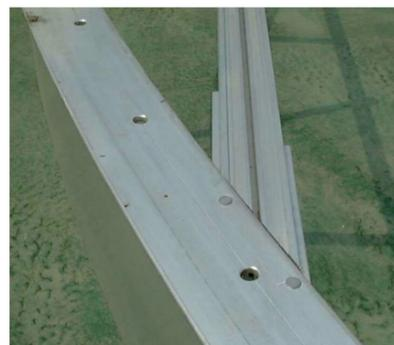
I-beam to rim bolted connection is strong and provides a continuous, flat surface for sheet clamping.
